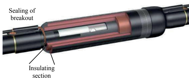
FIG. 7 Example of a heat shrink shield-break joint with sealed breakout integrated into the outer protection sleeve
