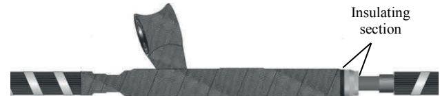
FIG. 8 Example of a cold shrink joint body with screen separation and copper mesh connected to the left side of the cable screen
