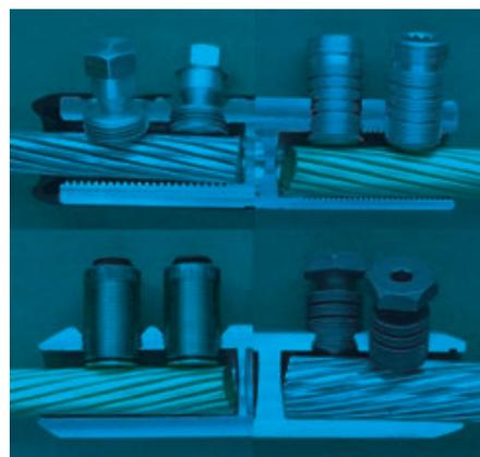
**Bolt design and material:** The bolt design is very important for the reliability. Different manufacturers have different designs to achieve this consistency in performance and each with patent protection. That's why there are a large number of different bolt designs in use. Most of these bolts are shear bolts with a special construction to guarantee no excess length over the outer.
