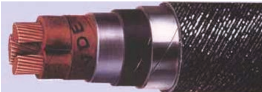
Figure 1 – 12 kV ‘belted’ paper-insulated cable with overall lead sheath and steel tape armour
