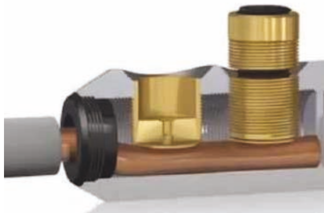
Figure 41 – Plastic insert (black) for centring a small conductor in the connector body
