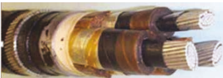
Figure 2 – ‘H’ type or ‘screened’ 36 kV paper-insulated cable with overall lead sheath and steel wire armour
