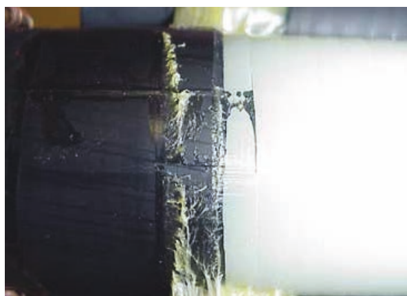
Figure 29 – Incomplete removal of conductive screen material from insulation surface
