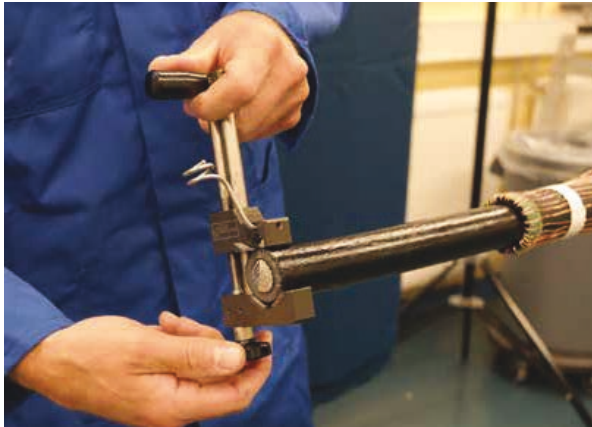
Figure 23 – Setting the correct cutting depth etc at the cable end (if no spare cable is available)
