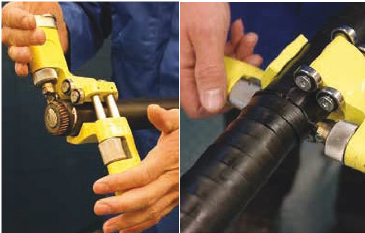
Figure 16 – Using a sheath removal tool
