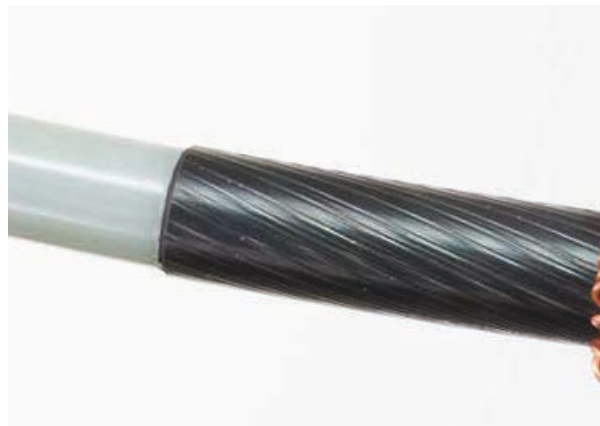
Figure 22 – Finished screen edge and smooth insulation surface
