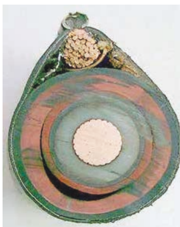
Figure 47 – Air void between layers of a heat-shrink joint
