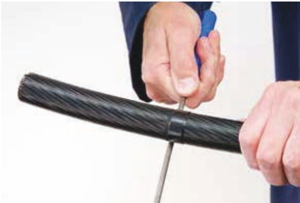
Figure 19 – Using a round file to create a screen edge
