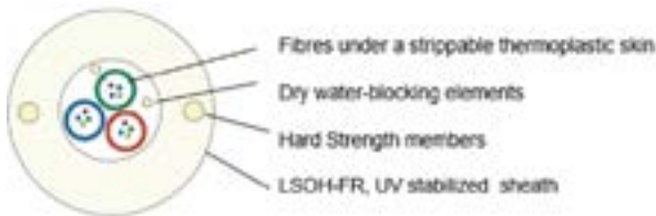
Figure 10 - Pushable round cable. Embedded strength elements in the jacket provide appropriate stiffness for pushing.
