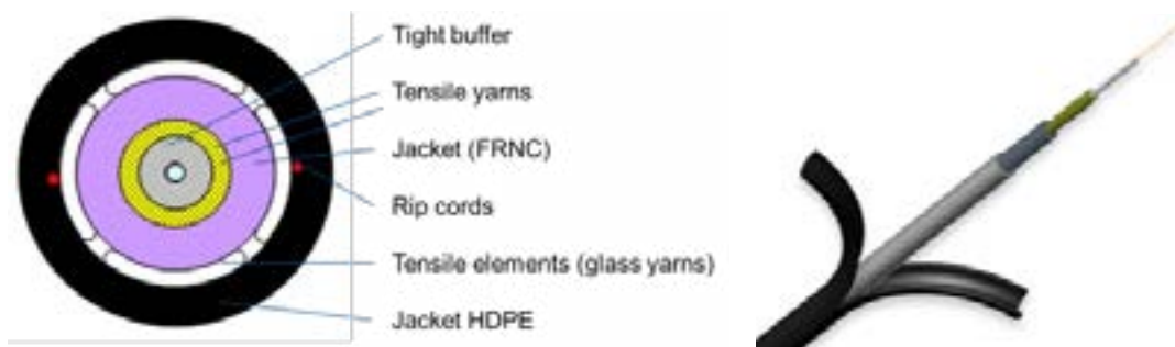
Figure 6a – Indoor / outdoor aerial drop cable with removable sheath. Alternate design with micromodule instead of Tight buffer are widely use.
