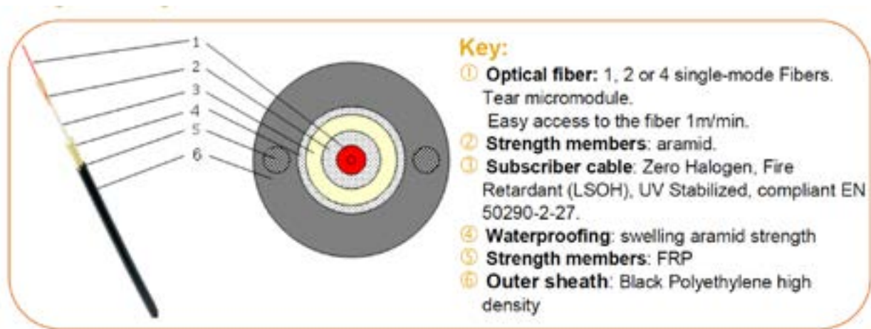
Figure 6b – Indoor / outdoor aerial drop cable with removable sheath.
