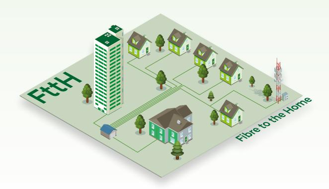
The passive infrastructure represents more than 80% of the overall cost of an optical fibre network and needs to be operational for several decades. This infrastructure is made up of a wide variety of equipment with very specific implementations:
